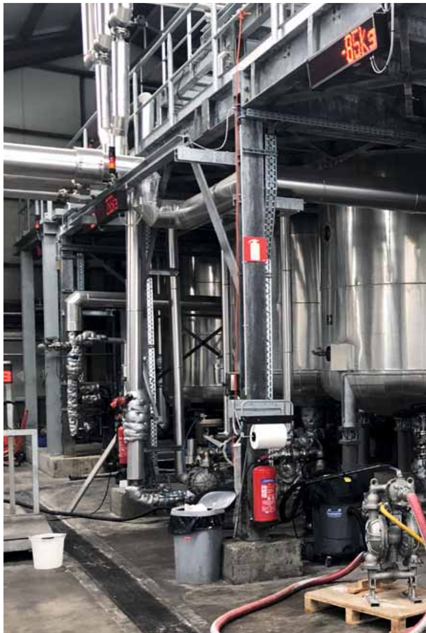
THERE ARE THREE 15M 3 STAINLESS STEEL REACTORS AND ONE 10M 3 HEAVY DUTY REACTOR AVAILABLE.
